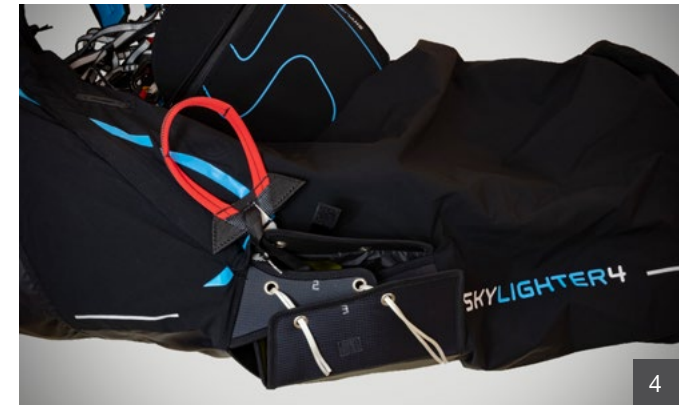
4 Using the lines provided (located in the rear pocket), thread the eyelets in sequence.
